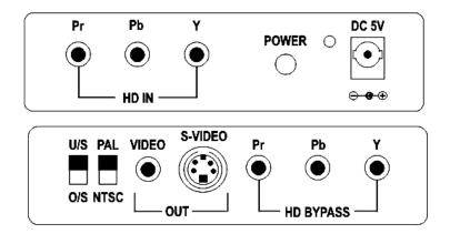
The NTSC/PAL switch on the output panel of the VS-223 allows selection of the desired television standard. The U/S – O/S switch allows selection of Underscan or Overscan video output.
