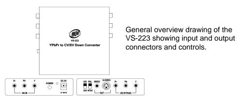
The input panel on the VS-223 is where the YPbPr input connectors are located. The Power Connector, Power Switch and Power "On" LED devices are also located on the input panel.
