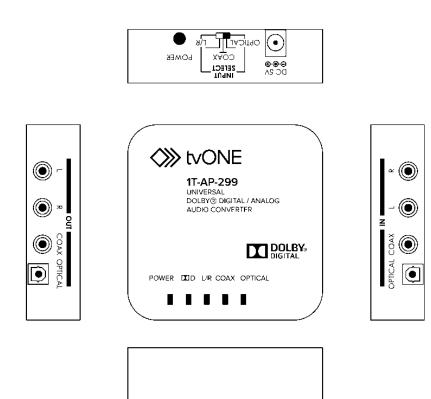
Connect the Output(s) from the source equipment to the appropriate Input connectors on the 1T-AP-299. Next, connect the 1T-AP-299's Optical, Coaxial and/or analog L and R outputs to the destination audio equipment. Set the Input Select Switch on the side of the 1T-AP-299 to the desired audio input mode (Optical, Coax or L/R).
