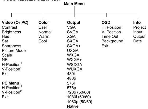
Note 1: The PC sub-menu is only visible when you have selected PC as your source. Note 2: H-Position and V-Position are only available when PC mode is selected.
