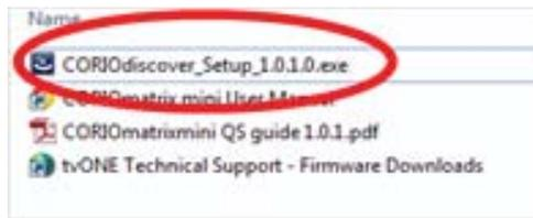
As well as installing the CORIOdiscover application, make sure your computer and the CORIOmatrix are on the same Ethernet network. If you do not want the CORIOmatrix on your network yet, you can connect the computer directly to the CORIOmatrix via Ethernet and configure it with this direct IP connection.
