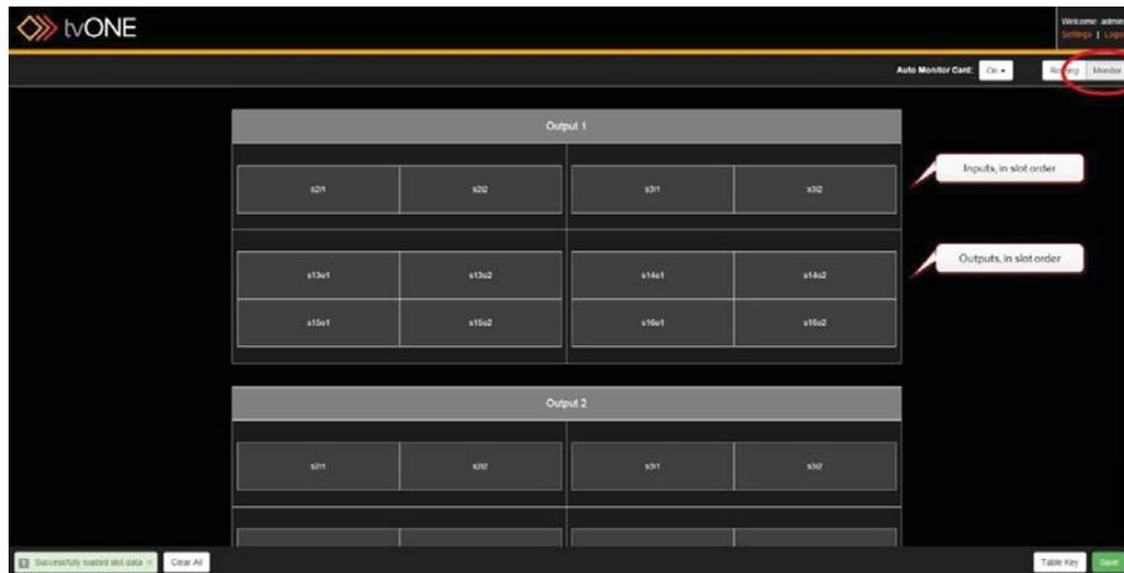
When the CORIOmatrix is in use, each small rectangle shows the video going through that input or output, and small green lines in the bottom left corner show audio channel activity.
