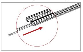
2. Work from the rear of the chassis. Position the lower rail with the numbers facing upwards and the M3 bolt strip facing outwards. Use four M4 screws to connect the rail to the side panels.
