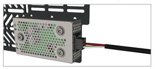
3. Connect the service cable to the internal power supply, or dual-redundant PSU.
