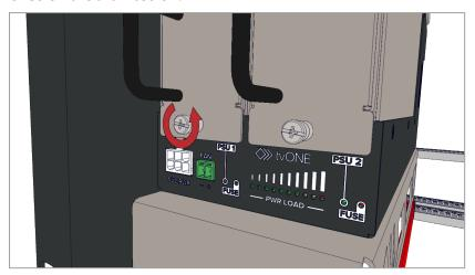
2. Use the handle to pull the power unit toward you and out of the dual-redundant PSU.
