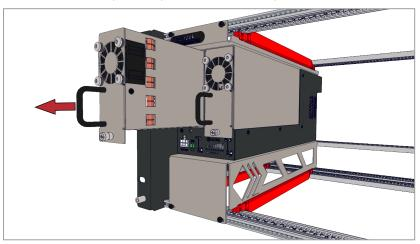
3. Slide the new power unit firmly into the dual-redundant PSU.
