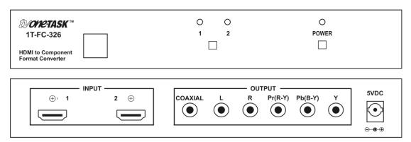
Connect the included AC adapter to a functional AC wall socket and then to the 1T-FC-326 Format Converter. Next, turn off any equipment intended to be connected to the 1T-FC-326 and, using high quality cables, connect the external equipment to the unit's inputs and output. Verify that the cables are fully seated in their respective connectors.
