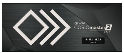
The front panel of your CORIOmaster2 LITE includes a customizable status screen. The status screen can show the IP address of your CORIOmaster2 LITE, its status, and the name of the device.
