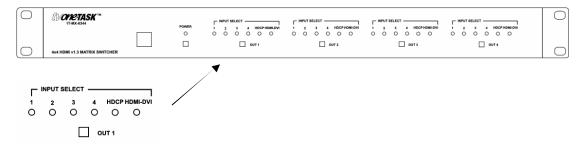
Decide on an output (1 through 4) and repeatedly press the small button associated with that output as shown in the example above to select the input. LEDs will illuminate as you step through the possible inputs, showing the input number you have selected. When you arrive at the input you wish to associate with the selected output, merely stop pressing the button.
