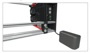
12. Plug the power lead into the mains supply.
