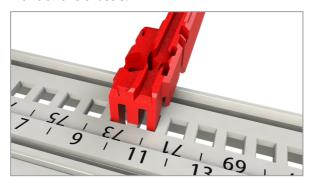
2. Slide the module into the groove in the guide rails.
