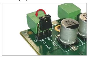
Any power connected to the voltage selector now bypasses the voltage selector switch.
