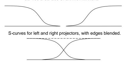
S-curves, when properly overlapping, will add together to result in full brightness.
