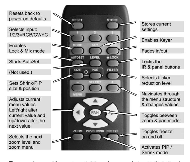
The transmit range of the remote control depends on many factors, but is designed to be fairly directional. Therefore you should always aim it directly towards your unit.
