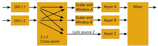
As the diagram shows, the two DVI-I inputs are available for use by either of the scalers, or as a lock source, also known as window Z, where the output is synchronized to an input.
