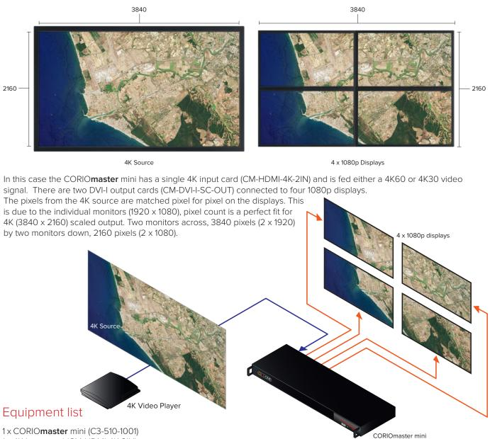
1 x 4K Input card (CM-HDMI-4K-2IN) 2x DVI-I Output cards (CM-DVI-I-SC-OUT) 4x 1920 x 1080p monitors, cables and mounts 1 x 4K source player and cables Computer with current Windows operating system and network cable for setup and system programming.
