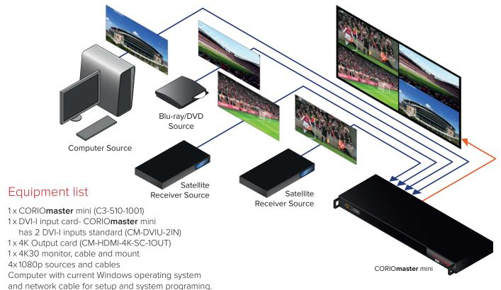
Additional 4K and HD inputs, windows and outputs can be added to the system to enhance your videowall arrangement. Up to four videowalls can be controlled by a single CORIOmaster unit. Let your creativity flow to build your visual experience.
