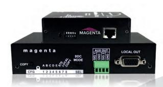
The MultiView II T4 (shown above, bottom) transmitter and the MultiView II STx (above, top) transmitter, in addition to gaining improved sync control and other MultiView II improvements, also add various EDID and DDC modes of operation, which their predecessors did not feature. These enhancements make it even easier to distribute 1080p (and higher) video to distances of 1,200 feet/366 meters.
