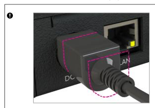
The power connector is a latching power connector. To remove the power connector from your Encoder-100, slide the sleeve backward.
