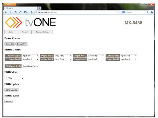
Note: The current IP address of the unit can be obtained from the LCD menu on the front panel.
