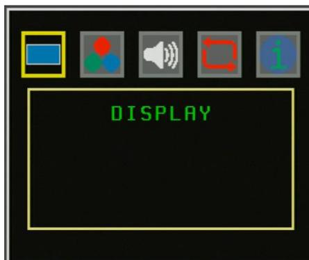
Use the + and – buttons to move horizontally across the first tier selections until you arrive at the one associated with the parameters you wish to adjust and then press the Enter button to select that parameter.
