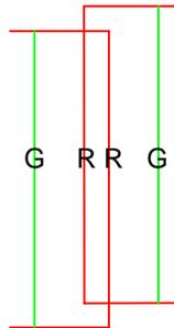
Offset – make sure your projectors are perfectly aligned both horizontally and vertically.
