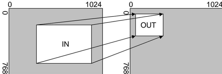
In the example above, 'In' has been set to 300,150 as its top-left source co-ordinate, with a size of 750,400. 'Out' has been set to 50,50 (i.e. close to the top left) with a size of 250,300.
