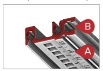
Use M4 screws to connect the rails to the side panel.
