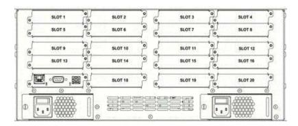
INPUT cards are painted black with white writing. They are placed in the unit from slot 1 onwards. The top row can only be inputs; remaining rows can be either inputs or outputs. Best practice is to add inputs in a left-to-right, top-to-bottom direction, while putting the first output card in slot 16 and working backwards.
