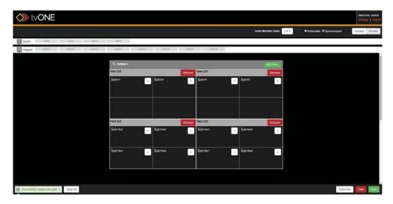
There are two outputs, to match the two output connectors on the monitor card. By default, the second output display duplicates the first. If you wish to use both output displays with unique content, uncheck the box and configure the second output appropriately.
