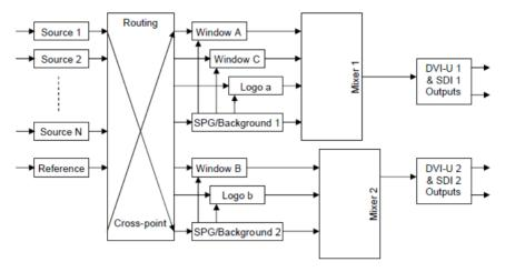
In the diagram above, the Windows are used for either Output 1 or 2, but never used on both. This allows the Sync Pulse Generators (SPGs) to run at different resolutions. Output 1 shows Windows A and C, whilst Output 2 shows Window B.
