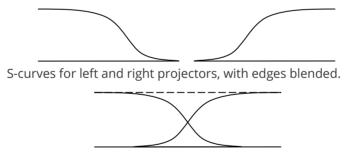
S-curves, when properly overlapping, will add together to result in full brightness.
