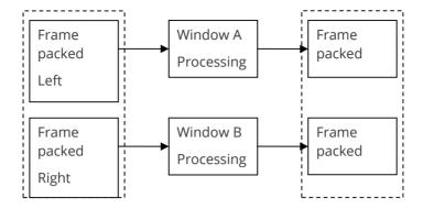
Along with the resolution scaling shown above, a scaler can be dedicated solely for use with each Left and Right image. This allows the 1080p 3D frame-rate conversion to be possible:
