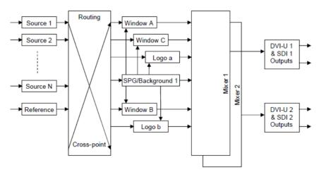
In the diagram above, all Windows are used for both Outputs 1 or 2, as both outputs are tied-together from the source sync source (and are thus always at the same resolution).
