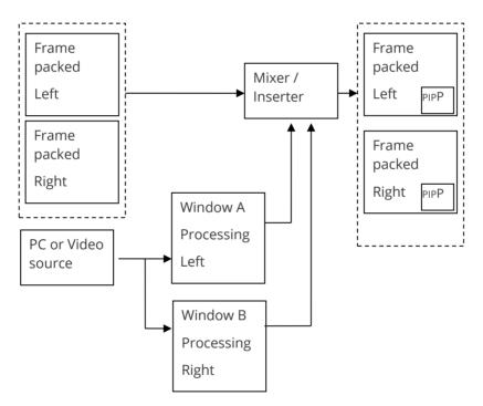
In order to achieve this, the CORIO2's 'LockandMix' mode is required, so that the background Frame-packed 3D source can pass through untouched – except for the insertion of the extra 2x PIPs from the scalers.
