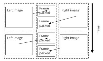
Because the video pixel rate has to be doubled in order to fit twice as many frames in during the same amount of time, only resolutions that are of low enough pixel rate can be doubled and still be within the DVI / HDMI pixel rate limit. These are:
