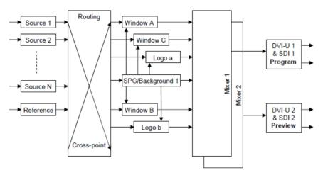
In the diagram above, the Preview output uses Window B (that is hidden from the user in the menu system) to show the next source and window size. On a transition, Window B is used to transition-in the new source before Window A shows it – thus allowing for a cross-dissolve to occur. Window C is shown on both outputs simultaneously.
