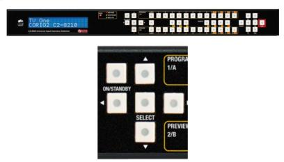
The crosshair (up/down/left/right) buttons on the front panel provides the user with a way of navigating the Liquid Crystal Display menus (LCD) which is detailed in a later section. Pressing and holding the ON/STANDBY button will place the unit into a low-power mode. A single press will turn it back on again.
